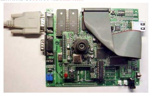
④ Connect 386EVB's U18 to PC's NIC(Network Interface Card,LAN card) with UTP cable(Cross cable)
